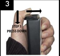
With the keypad facing away from you, close the cover by gently pressing it down (STEP 1) and sliding it until it aligns with the front (keypad) of the device (STEP 2).
